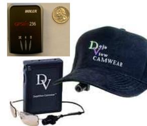
Small wearable devices for capturing context: GPS receiver (top) and Camera (bottom), which can be mounted on hat or eyeglasses
